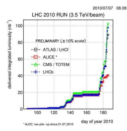
They have now switched from a 7 bunch filling scheme to 10 bunches per beam. The number of collisions per turn is still four so the luminosity will not improve, but this new scheme should have less problems with interactions between bunches. This will mean better stability and longer runs if they can avoid other hitches.
