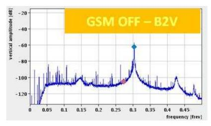
The Hump takes the form of a hump in the spectrum of beam oscillations that drifts up and down the frequency range. The beam is normally given a tune frequency away from any interference to keep it stable, but because the hump frequency keeps changing it is difficult to avoid whatever tune frequency is chosen.
