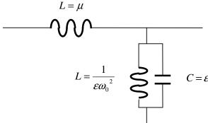
The transmission line is dispersive because the characteristic impedance (29) is frequency dependent and it resonates when:
