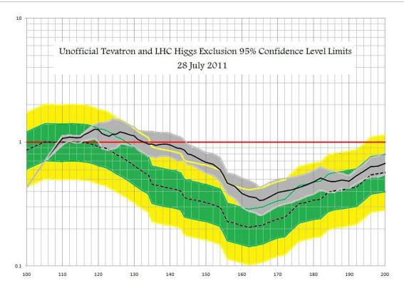
What this is showing is that an excess around the 140 GeV area is possible but it is not likely to be consistent with a standard model Higgs because it is below or near the red line. We can strengthen this by doing the global fit with the combination uncertainty shown. The electroweak precision tests reduce the likelihood that a Standard Model Higgs Boson is at this mass.
