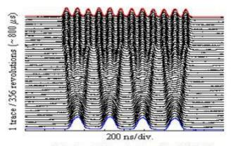
Splitting of 4 bunches into 12 at 1.4 GeV.
