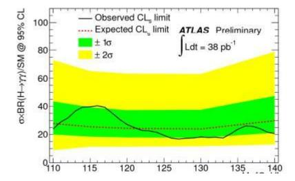
All these plots show a small excess around the 110 GeV - 120 GeV region, but the size is not significant and the positions are not quite consistent. Will we look back on these graphics in a few months time as the first signals of the Higgs or as statistical flukes?
