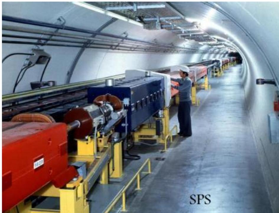
Now the SPS is the final stage that injects the protons into the Large Hadron Collider. Since it is more than ten times as big as the PS it can easily build up much larger trains of protons by collecting together the trains of bunches fed from the PS. For the fill running now it takes three trains of 36 bunches from the PS one at a time to form trains of 108 bunches to feed into the LHC.
